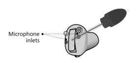
Clean the vent by pressing the brush through the hole while twisting it slightly.
