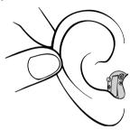
Gently pull your ear outwards and push the hearing aid into the ear canal, twisting slightly if necessary. Follow the natural contour of the ear canal. Push the hearing aid to make sure it fits comfortably in the ear.
